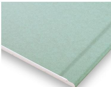
**Product description:** Gypsum plasterboard acc. to DIN EN 520, type DFH2, moisture-resistant, made of a special, reinforced gypsum core encased in cardboard.
