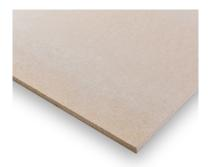
**Product description:** Homogeneous gypsum fibreboard with square edges (SK). Pre-primed, smooth and extremely hard surface. Fire rating class A1. U.S. Coast Guard and notified body approval 164.109/EC0736/107.088/EC0045. **Area of application:** Suitable for marine ship interior application.
