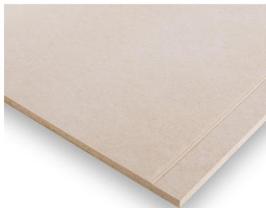
**Product description:** Homogeneous gypsum fibreboard with tapered longitudinal edgess (AK). Pre-primed, smooth and extremely hard surface. All characteristic values for the design in timber construction are deposited in ETA 08/0147
