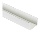
Product description: Metal stud according to DIN 18182-1 / DIN EN 14195 made of sheet steel according to DIN EN 10346 with a coating according to DIN 55634. Material tolerances according to DIN EN 10143. Corrosion category C3high / C4-high according to DIN EN ISO 12944.
