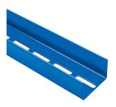
Product description: Metal stud according to DIN 18182-1 / DIN EN 14195 made of sheet steel according to DIN EN 10346 with a coating according to DIN 55634. Material tolerances according to DIN EN 10143. Corrosion category C3high to C5-high according to DIN EN ISO 12944.
