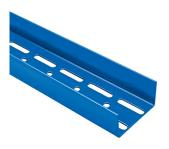
Product description: Metal stud according to DIN 18182-1 / DIN EN 14195 made of sheet steel according to DIN EN 10346 with a coating according to DIN 55634. Material tolerances according to DIN EN 10143. Corrosion category C3high to C5-high according to DIN EN ISO 12944.
