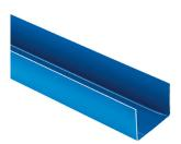
**Product description:** Metal stud according to DIN 18182-1 / DIN EN 14195 made of sheet steel according to DIN EN 10346 with a coating according to DIN 55634. Material tolerances according to DIN EN 10143. Corrosion category C5-high according to DIN EN ISO 12944.
