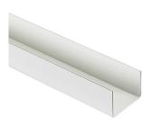
**Product description:** Metal stud according to DIN 18182-1 / DIN EN 14195 made of sheet steel according to DIN EN 10346 with a coating according to DIN 55634. Material tolerances according to DIN EN 10143. Corrosion category C3-high / C4-high according to DIN EN ISO 12944.
