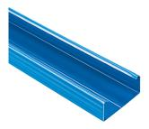
Product description: Metal stud according to DIN 18182-1 / DIN EN 14195 made of sheet steel according to DIN EN 10346. Material tolerances according to DIN EN 10143. Corrosion category C5-high according to DIN EN ISO 12944.
